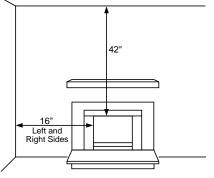
Figure 4 - Minimum Clearance to Wall and Ceiling
